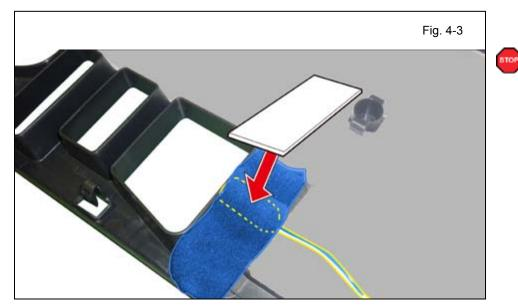
d. Apply 1 Foam Tape to the GBS Microphone as shown.
